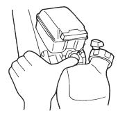
Move the choke lever upward to choke position.
