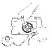
Lubricate the recoil spring with light oil. Fit the cassette with recoil spring in the starter. Fit the starter pulley and tension the recoil spring.
