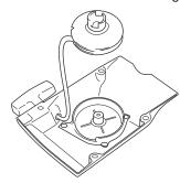
Remove the recoil spring from inside the pulley by tapping the pulley lightly with its inside face downwards against a work bench or the like. If the spring pops out during fitting, wind it up again, working from the outside in towards centre.
