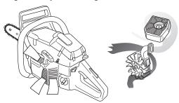
IMPORTANT! In order to maintain operation of the centrifugal cleaning system it must be regularly maintained. Clean the air intake to the starter, the fins on the flywheel, the space around the flywheel, inlet pipe and carburetor compartment.
