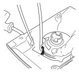
• Undo the screw in the centre of the pulley and remove the pulley. Insert and fasten a new starter cord to the pulley. Wind approx. 3 turns of the starter cord onto the pulley. Connect the pulley to the recoil spring so that the end of the spring engages in the pulley. Fit the screw in the centre of the pulley. Insert the starter cord through the hole in the starter housing and the starter handle. Make a secure knot in the end of the starter cord.
