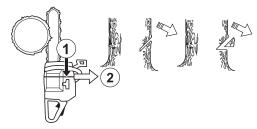
The directional cuts should run 1/4 of the diameter through the trunk and the angle between the top cut and bottom cut should be 45°.
