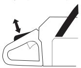
Check that the throttle control and throttle lockout move freely and that the return springs work properly.
