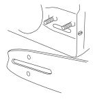
Tension the chain by turning the chain tensioning screw clockwise using the combination spanner. The chain should be tensioned until it does not sag from the underside of the bar.
