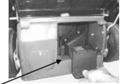
Figure 10. Mulch plug installation (B) - Self Propelled Mower
