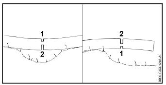
If the limb is under tension: Make the relieving cut (1) at the compression side and then perform bucking cut (2) from the tension side.
