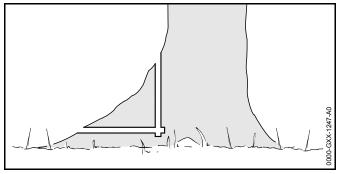
If the tree has large, healthy buttress roots: Make vertical cut first and then a horizontal cut, and remove the resulting piece.
