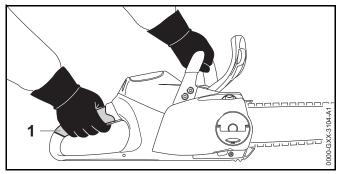
Hold and control your saw with your left hand on the front handle and your right hand on the grip area (1) of the control handle. Wrap thumb of left hand around the front handle and thumb of right handle around the control handle.
