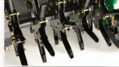
Standard ¾", austemper-hardened steel coring tines stand up to the daily rigors of even the most difficult jobs.
