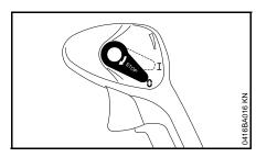
Push the setting lever in the direction of 0 – the engine stops – the setting lever then springs back automatically.
