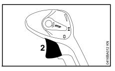
Blip the throttle trigger – the choke knob automatically returns to "I"
