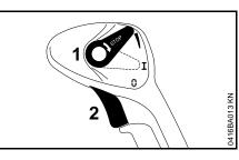
The throttle trigger (2) can be locked in any position.
