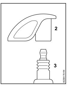
Screw the spark plug (3) into the cylinder and fit the boot (2) (press it down firmly).
