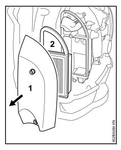
• Remove the filter cover (1) and air filter element (2).
